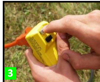
3 PRESS "TEST" BUTTON TO VERIFY GFI FUNCTION, THEN PRESS "RESET"
