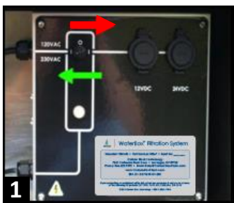
1 SWITCH TO LEFT FOR AC POWER SWITCH TO RIGHT FOR DC POWER SWITCH TO CENTER FOR OFF
